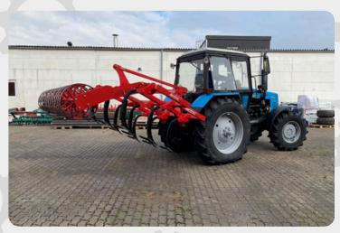
Heavy stubble cultivator with two types of rollers and a complete second set of working tools.
