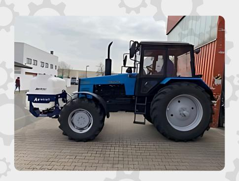
600-liter tank with an electric drive and dosage regulation for applying liquid fertilizers. With a front mount on the front of the tractor.
