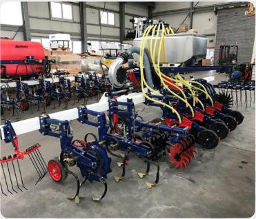
A universal frame with a three-point hitch and two adjustable support wheels as the main carrier. Possible configuration from 2.5m to 12m.
